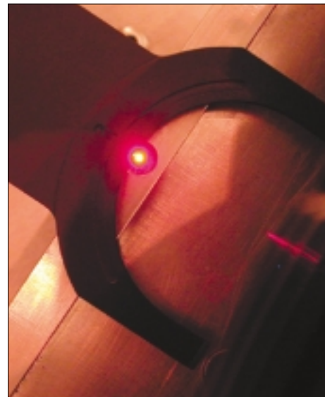
Robot end-effector cutting through-beam optical sensor path
