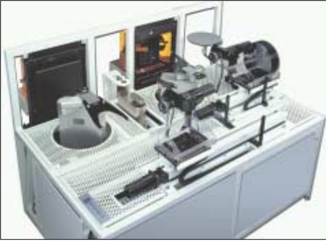
Figure 6: The 300-mm wet bench (illustrated in Figure 5) with the single-controller architecture.
